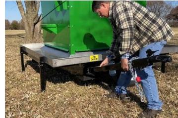
**Step 6 - Open the feed shut off gate by pulling the handle all the way out and down to secure**
