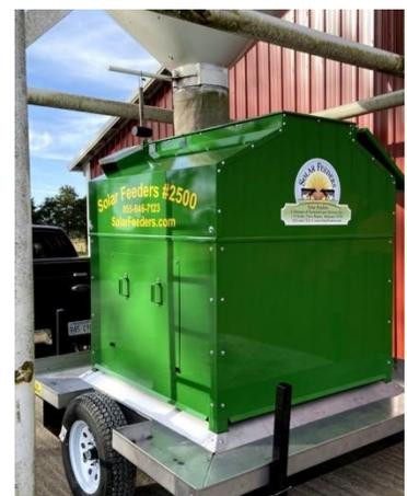
**Step 4 – Tow to feeding area and position on a level surface, securing the four stabilizing legs (one in each corner)**
