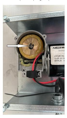
If snap ring and gear/shaft assembly are intact then proceed to replacing the motor.
