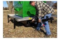
Step 6 - Open the feed shut off gate by pulling the handle all the way out and down to secure
