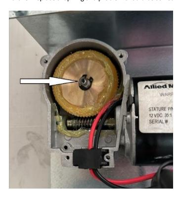
If snap ring and gear/shaft assembly are intact ONLY then proceed to Replacing the motor.
