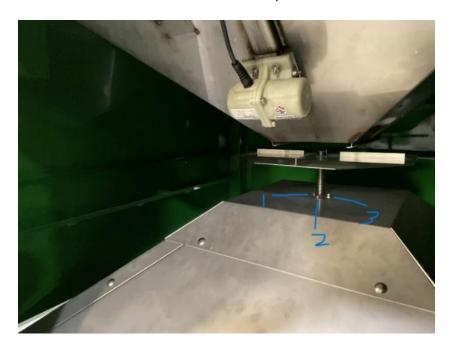
Remove the threaded shaft from the motor shaft (see illustration below) by loosening the set screw with a 1/8 hex key drive (allen wrench) and then use a small punch to remove the roll pin.
